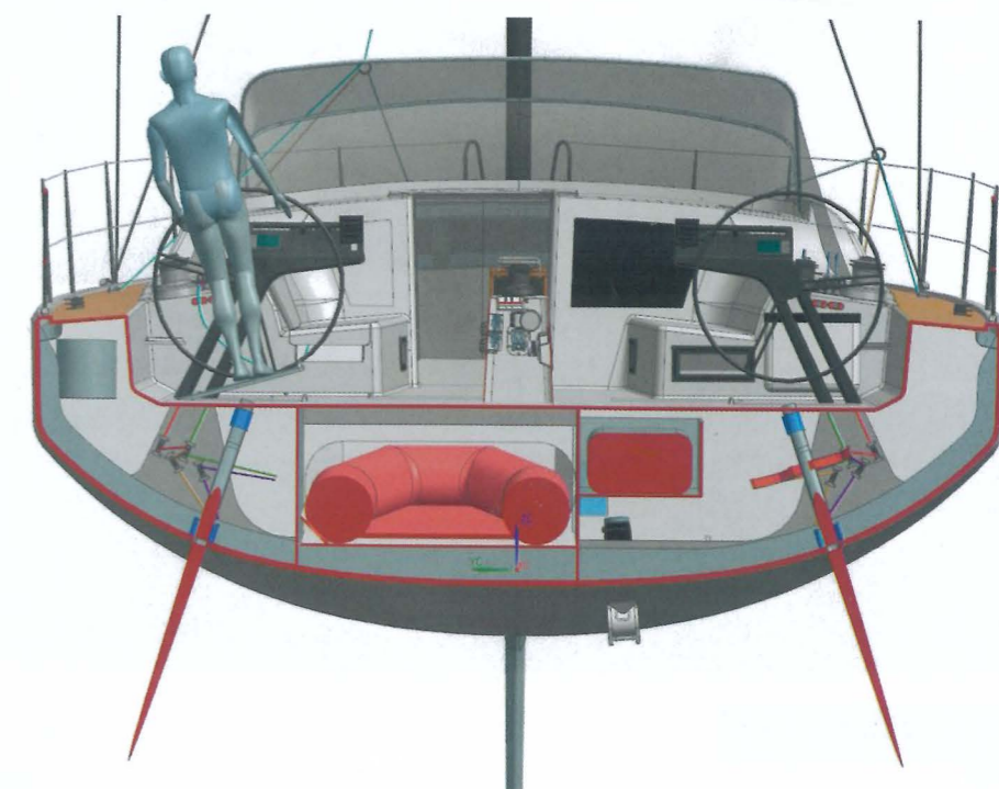
With 5.26m of beam, there is room in the transom for a dinghy. The garage is slightly offset, with space at the side for dedicated liferaft stowage
